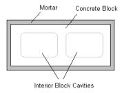
Figure 1: Construction of Typical Concrete Block
